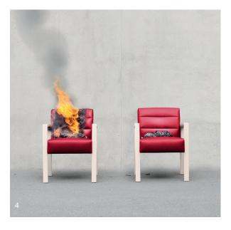
**5** The key to effective fire prevention is a special upholstery compound with a non-combustible glass fabric (A2) compliant with DIN 4102 between the flame-protected foam and the upholstery cover. This separating layer prevents fire on the upholstery cover from spreading to the upholstery foam for a specified amount of time – incidentally, additional, ecologically questionable flame retardants are not needed. Photo: Kusch+Co
